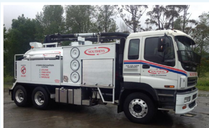
Figure 1 Vacuum truck or hand digging to identify and avoid underground services
